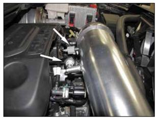
12. Connect the crank case vent line and inlet air temperature sensor electrical connection.
