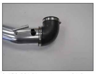
10. Install the inlet air temperature sensor into the SPECTRE® intake tube using the provided grommet. Install the 90° coupler onto the SPECTRE® intake tube and secure with the provided hose clamp.
