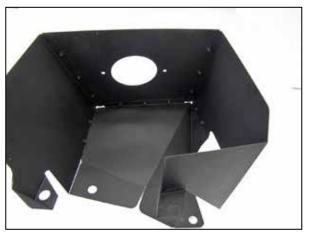
4. Assemble the four panels of the heat shield using the provided hardware.
